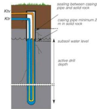
*Fig. 6.5 - Typical Closed loop Bore hole arrangement.*
