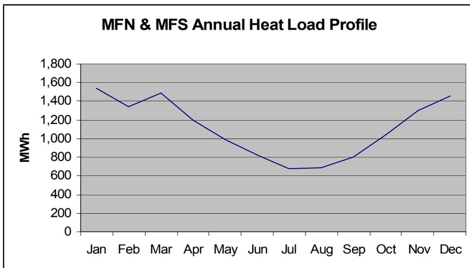
7.28 It has been estimated that the CHP engine runs for 20-24 hours per day during the winter periods and approximately 8-15 hours during the summer periods, as illustrated in the diagrams below, this equates to 6,350 hours per year. A series of thermal stores will be installed to store excess heat produced during times of low hot water demand (e.g. between 11pm and 6am) for later use.
