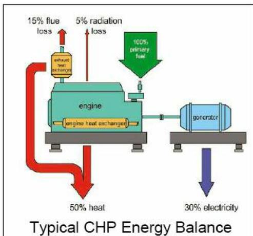
*Fig 7.1 – Typical CHP Energy Balance*
