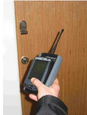
These meters have the facility to send a radio signal output to a hand held PDA unit to collect the data for management billing. This will enable the facilities management company to collect an entire buildings energy data from one single point – (externally to the building) without unnecessary access to each unit.
