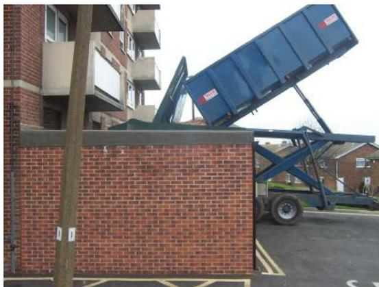
*Fig 6.4 - Delivery of biomass fuel by tipping*
