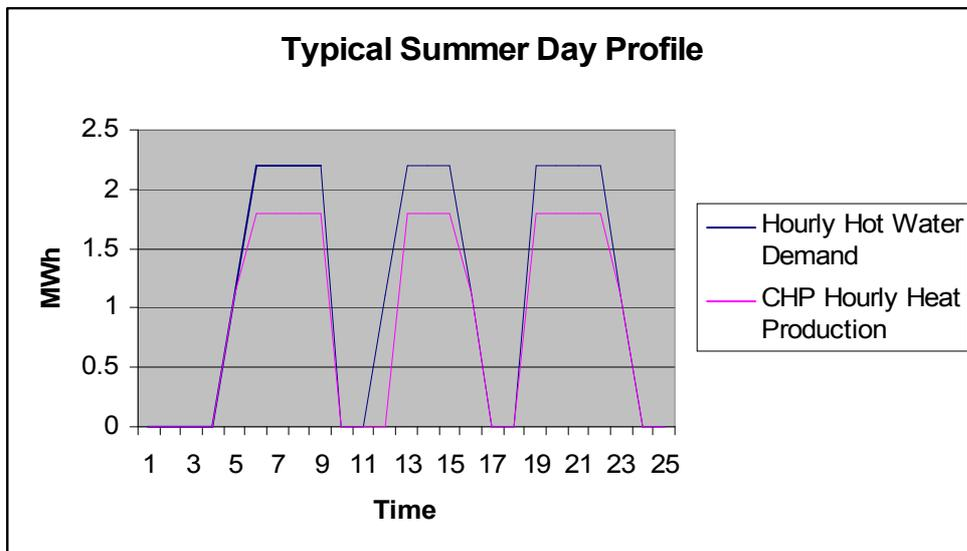
7.29 The CHP will be the lead boiler for heating and DHW to meet the baseload demand. However, the CHP boiler will only be capable of providing part of the peak instantaneous load. Additional demands for heating will be met by the new gas-fired boilers, sequenced to come on only when the demand is greater than the CHP can provide. There will be no direct electric heating. The diagram below indicates the CHP
